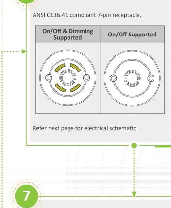
For installation, place the WALI Node firmly into the ANSI C136.41 compliant 7-pin receptacle and twist clockwise until it locks into place.
