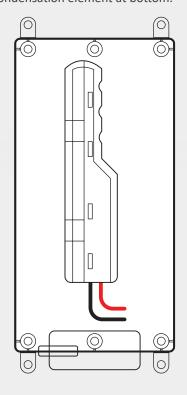
Use an inside the box drip-deflector to divert any condensation that forms inside the box away from the wireless device, or drill a couple of small holes on the bottom side of the enclosure to allow condensation to drain accordingly.
