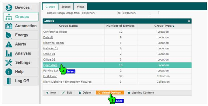
5. The Virtual Devices: Open area window appears, click on the New button to create a new Virtual Device.
