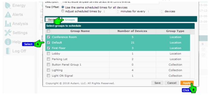
• The **Time Offset** feature is typically used in HVAC applications. Device start times can be staggered to mitigate electrical surges.
