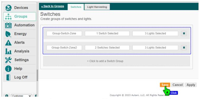
13. If necessary to delete any of the Switch Group select the "X" button, the respective switch will get deleted.
