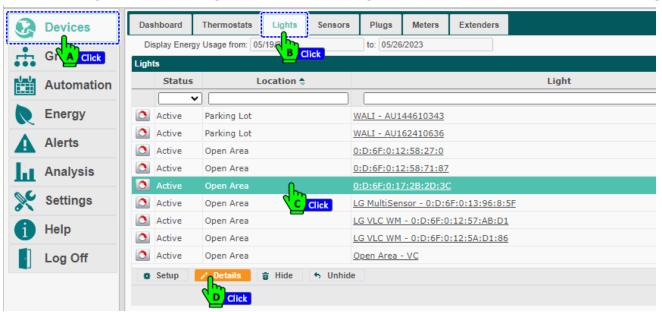
Select the sensors tab and associate the occupancy sensor/s to the light.
