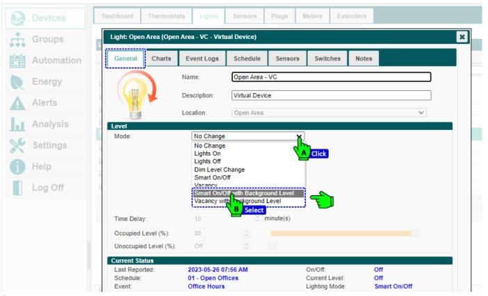
4. The settings for the "Smart On/Off with Background Level" is listed below the drop down. Change the settings accordingly per the requirement and click save. Each setting is explained below.
