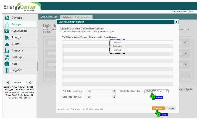
• The main reason to run **calibration** is to keep Light Value stable. And when the area is dark, Light Value will be most stable.
