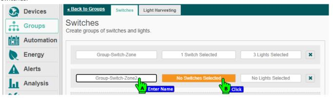
9. The select Devices window opens. Select the switch (in case of dimmer select two switches with same ID) and click "Select" button.
