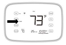
Figure 28. System mode is set to Heat
