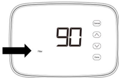
Figure 30. Filter reminder is on
