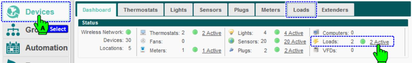
The Dashboard displays the number of active load controller relays in the system. To view additional detail on all relays, click the active status link next to the number of load controllers or click the **Loads** tab.
